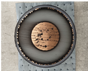
Fig. 1: Cross-sectional image of an underground high voltage cable
